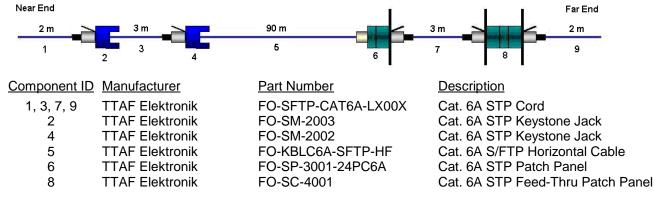
Standard(s)/Specification: ANSI/TIA-568-B.2-10 Category 6A with the applicable electrical transmission characteristics
